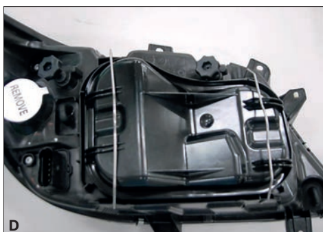
D Mount the cover and engage the spring.
