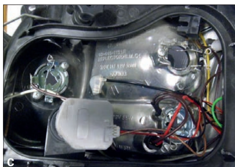
C Fit in the servo motor of the original lamp then assemble the harness.
