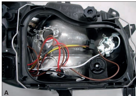
A Remove the spring and take out the cover.
