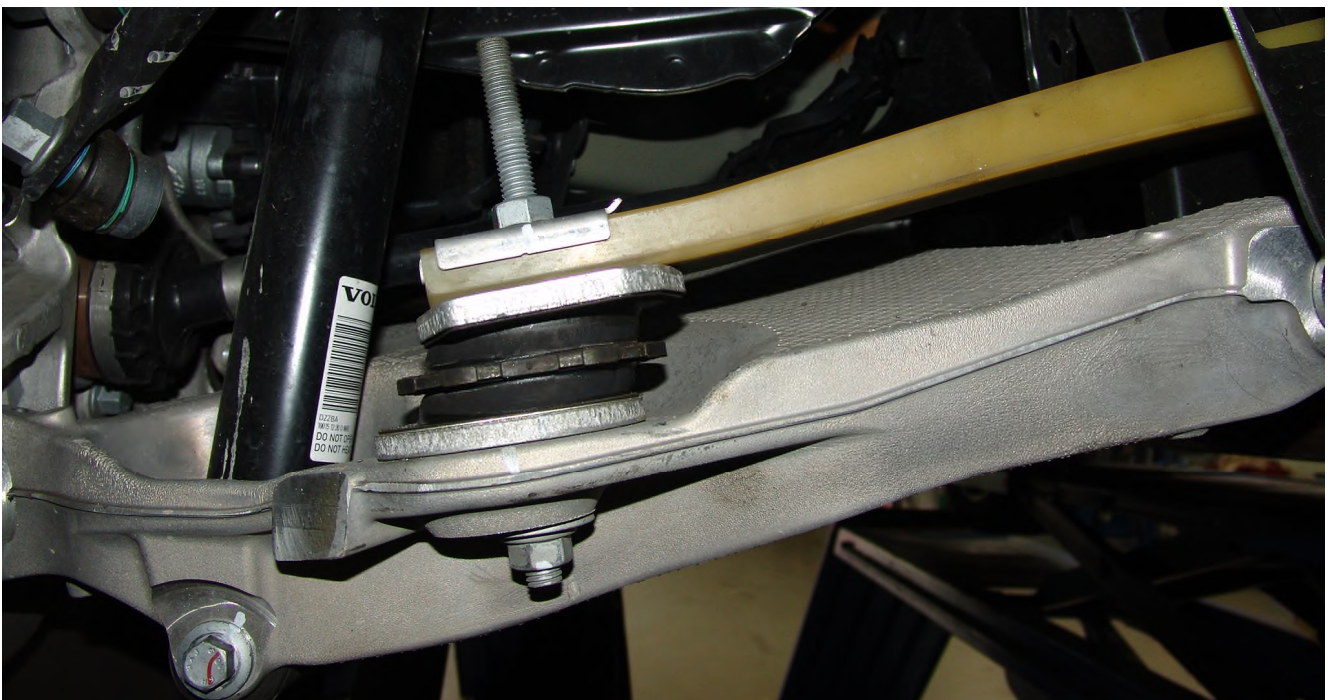
Illustration 2: removing the spring pad left and right
