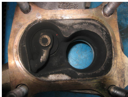
Gasket incorrectly mounted
