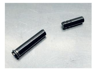
**Damaged internal element** Due to bad torque tightening of the injector.
