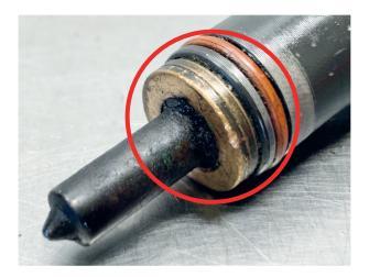
**Uncleaned contact area surfaces** Insufficiently cleaned and leveled.
