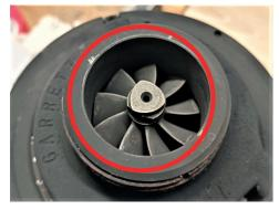
Insufficient oil supply to the turbocharger rotor – damage of the turbine wheel and turbine housing caused by axial or radial play due to insufficient lubrication of the turbocharger rotor.
