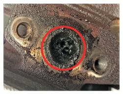
**Clogged oil flange –** carbonized oil particles from engine oil due to neglected maintenance. Excessive engine deposits or residual sealant.
