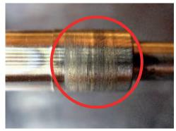
Insufficient oil supply to the turbocharger rotor – damage of the turbine rotor caused by insufficient lubrication.
