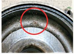
**Damaged compressor wheel flaps –** caused by particles in the intake due to impurities.
