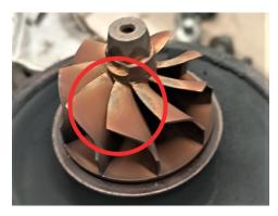
Burnt turbine wheel – in most cases caused by clogged DPF system.
