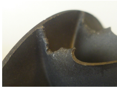
Damaged exhaust turbine
